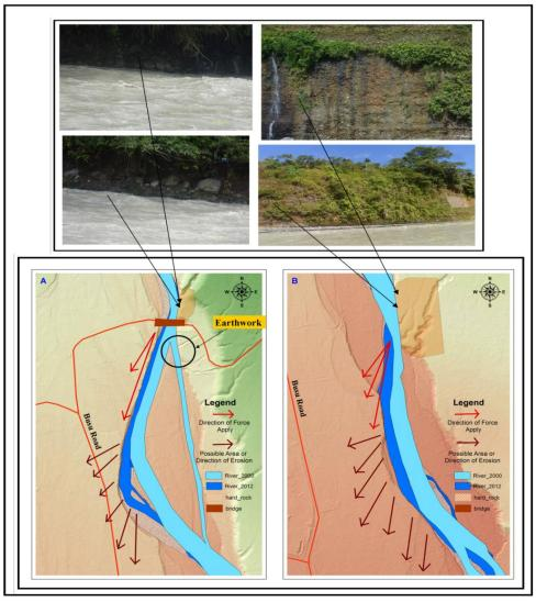
Figure 5: Possible direction of river force and erosion (Map A-LC1 & Map B-LC2) (Source: Author, 2016)
