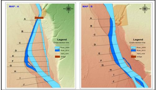
Figure 4: Cross-Section lines drawn to measure river shift and impact (Map A-LC 1 & Map B-LC 2) (source: Author, 2016)
